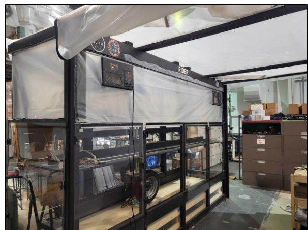
Figure 1. RIDER with road tire installed for system validation and testing (March 2023).
